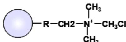
Fig.2 Ligand Structure of Cellufine MAX Q-hv
