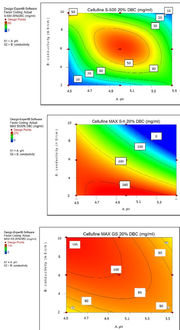
Figure 3: mAb DBC with Cellufine CEX resins
