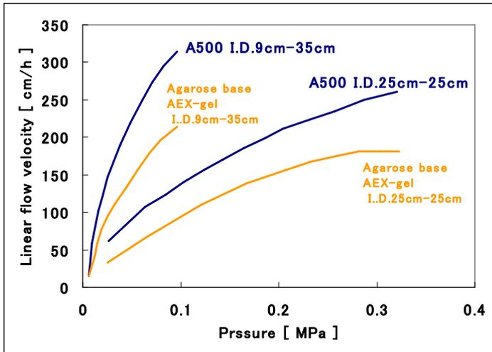
The flow/pressure curve for a Cellufine A-500 column confirms operating flow rates above 250 cm/h can be obtained at column size I.D.25cm.
