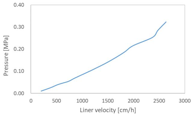
Fig. 3 Pressure-flow curve of Cellufine MAX Butyl HS
