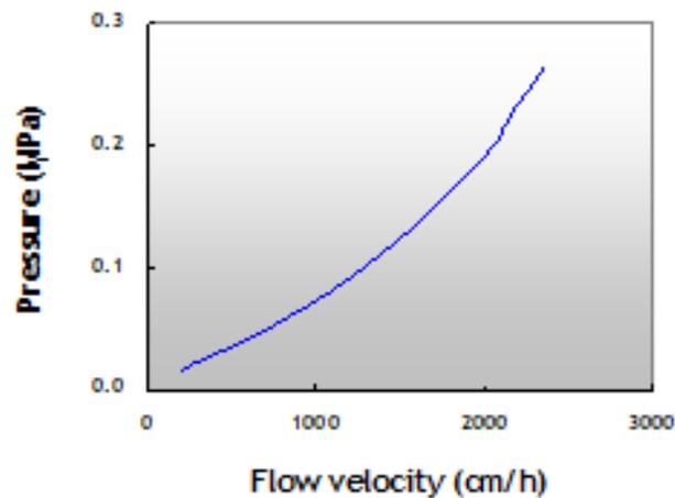
Column: 2.2cm Diam. x 20 cm L, Temperature: 24 $\pm$ 1  $^\circ\text{C}$ , Mobile phase: water
