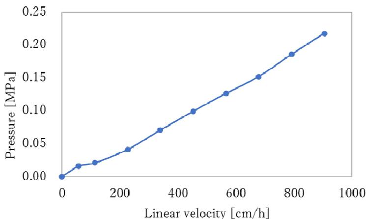
Fig.1 Flow property of Cellufine Phenyl EX
