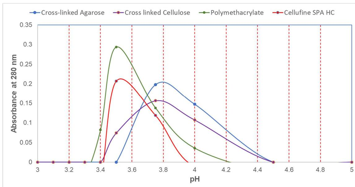
The above result shows that Cellufine SPA-HC and the polymethacrylate based resin both show peak elution at pH 3.5 and the other two resins at pH 3.8. This difference in elution pH presumably reflects the structure of the different rProtein A affinity ligands on these commercial resins. This methodology is a very quick way to screen elution pH and uses very little material.
