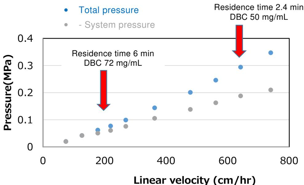
Pressure/Flow test was carried out in a 10 cmID x 20 cmL column (Axichrom 10/300, 1.57L CV, GE healthcare) with a water mobile phase at 20-25 °C.
