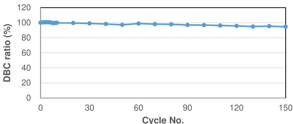
Figure 4 shows high retention (>95%) of DBC after 150 cycle 0.1M NaOH CIP. The capacity at cycle zero was 75 mg/mL and changed to 72 mg/mL at the end of the study.
