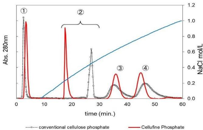
Fig.1 Separation of mixed sample
