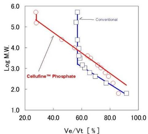
Fig.2 Cellufine Phosphate has a large pore compared with conventional Cellulose Phosphate.
