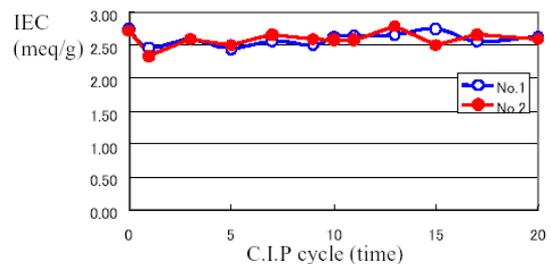
Cellufine Phosphate is stable to cleaning in place (C.I.P) by alkali.
