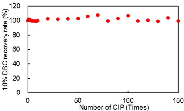
Protein recovery after multiple cycles of base CIP was measured in a 5 mmID x 2.5 cmL (volume 0.49 ml) flow packed column at a flow rate of 0.125 ml/min for a residence time of 4 min. Lysozyme at 2 mg/ml was loaded in a Buffer A; 50 mM Tris HCl pH 9.5 + 150 mM NaCl. Retained protein was recovered by elution with Buffer B; 50 mM Tris HCl pH 9.5 + 1.0 M NaCl.
