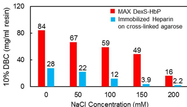
DBC was measured in a 5 mmID x 2.5 cmL (volume 0.49 ml) flow packed column at a flow rate of 0.125 ml/min for a residence time of 4 min. Lysozyme at 2 mg/ml was loaded in a 50 mM Tris
