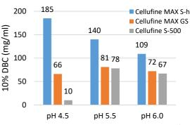
Adsorption condition; 10 mM Acetate (pH 4.5, 5 mS/cm) or 10 mM MES-NaOH (pH 5.5 and 6.0, 5 mS/cm) Residence time; 2 min
