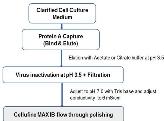
Loading buffer conductivities and elution buffer species (citrate and acetate) were evaluated in this study. Dextran modified anion IEX resins such as Cellufine MAX Q-h and a polymer modified Agarose-Q were used as reference. Samples for these resins were adjusted to the pH that matches the recommended flow through conditions for these resins. The results are summarized in Figure 3 below.
