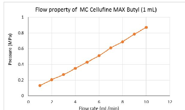
Mobile phase: pure water (23 °C), Measured without using restrictor.
