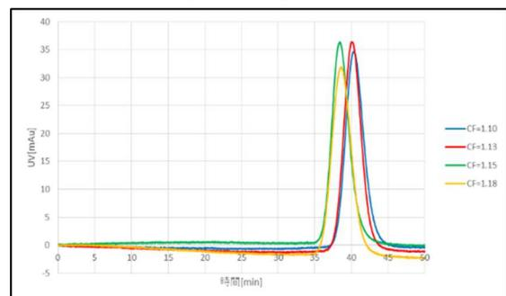
Table 4, Column packing efficiency data over a range of packing pressures
