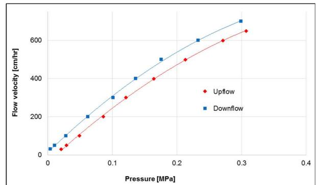
**Example of flow packing a 30 cm ID column with Cellufine MAX Q-h**
