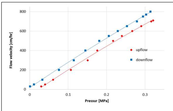
**Example of flow packing a 30 cm ID column with Cellufine MAX S-r**
