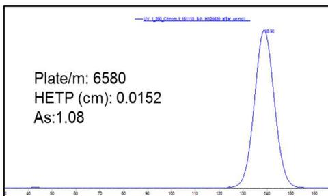
Post packing flow conditioning the 3.2 cm ID column did lead to a significant improvement in the number of theoretical plates/m and a very acceptable peak As of 1.08.
