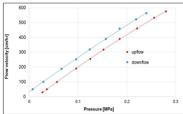
The above data shows that a 30 cm ID column of Cellufine MAX DEAE can be successfully flow packed with a compression factor in the range of 1.10 to 1.18 to yield a qualification peaks with a narrow As range of 1.09 to 1.18.
