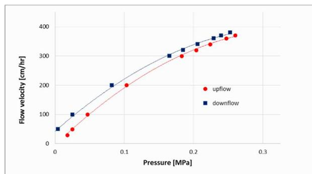
This data suggests that an optimal compression factor for packing Cellufine A-500 in a 30 cm ID column was 1.125 to 1.175. In Figure 4 above, a pressure - flow velocity curve of Cellufine A-500 packed in a 30 cm I.D. column is shown with flow in both directions.
