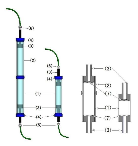
The Operating Instructions use a simple cross-sectional figure of the column, as shown on the right.
