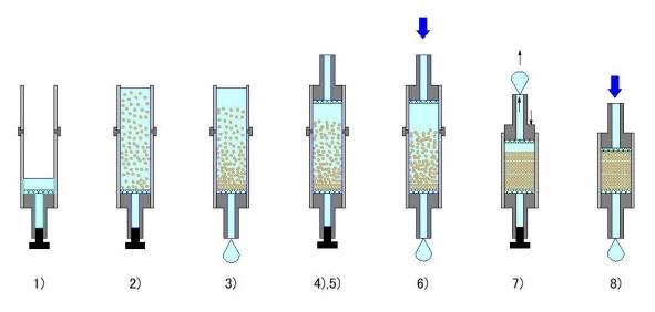
Figure 2 Process of column packing
