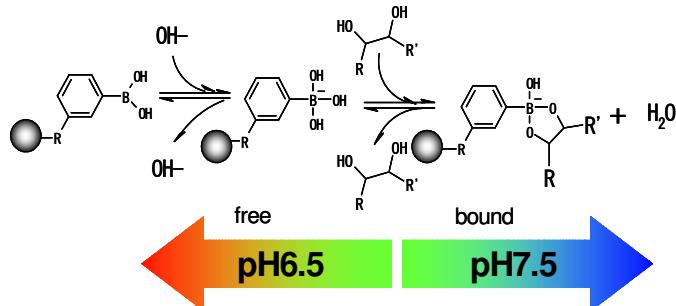
Adsorption and desorption mechanism of Cellufine™ PB
