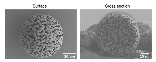
Fig.1. Cellulose resin MLP1000
