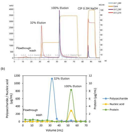
**Figure 3.** Experimentally obtained chromatogram of Cellufine MAX Q-hv (a) and the results of fraction analysis (b).
