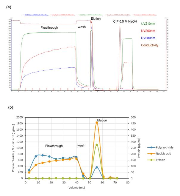
**Figure 2.** Experimentally obtained chromatogram of Cellufine MAX Butyl HS (a) and the results of fraction analysis (b).
