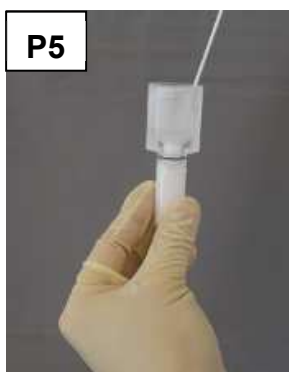
Photograph P5; using a pipette to remove excess slurry from the packing reservoir-column tube assembly.
