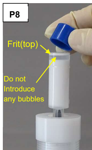
Photograph P8; assembly of the top blue cap on top of the frit and the settled bed in the column tube.
