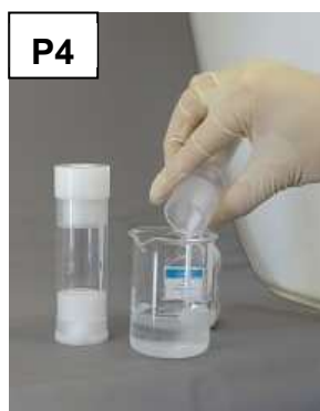
Photograph P4; pouring excess slurry from packing reservoir-column tube assembly.
