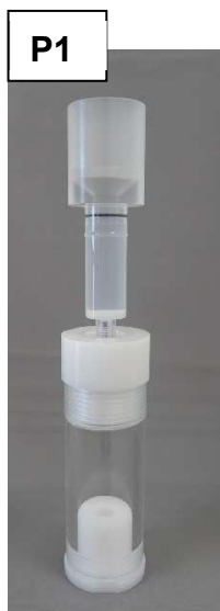
Photograph P1; 5 mL packing reservoir assembled on top of the column tube and supported in a vertical orientation in the screw press/stand.
