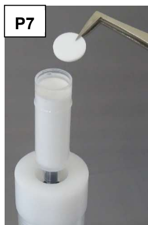
Photograph P7; adding the frit to the top of the column tube.
