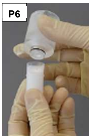
Photograph P6; Separation of the packing reservoir from the column tube.
