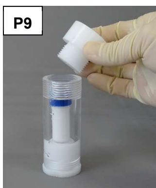
Photograph P9; Assembly of top screw and screw press/stand.
