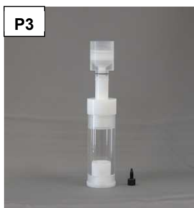
Photograph P3; allowing slurry to settle under flow in the packing reservoir-column tube assembly in the screw press/stand
