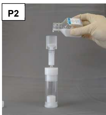
Photograph P2; adding slurry to the packing reservoir-column tube assembly in the screw press/stand.
