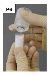
Photograph P6; Separation of the packing reservoir from the column tube.
