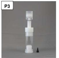
**Photograph P3**; allowing slurry to settle under flow in the packing reservoir-column tube assembly in the screw press/stand
