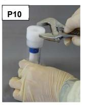
Photograph P10; Using an adjustable wrench to seal top screw
