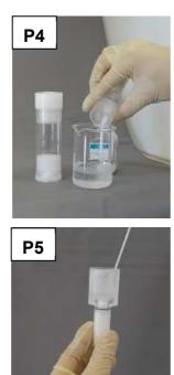
**Photograph P4**; pouring excess slurry from packing reservoir-column tube assembly.
