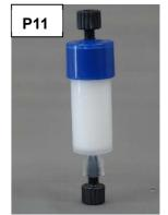
16) Install the stop plug at the top of the column cap (Photograph P11).
