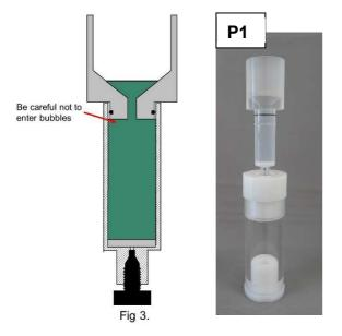
**Photograph P1**; 5 mL packing reservoir assembled on top of the column tube and supported in a vertical orientation in the screw press/stand. 5) Prepare a 50-70% slurry of the resin in 20% Ethanol and measure % solids by allowing the slurry to settle in a slurry bottle for a minimum of 4 h.
