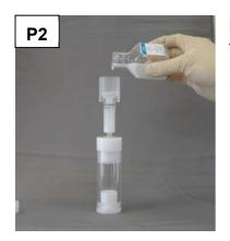
**Photograph P2**; adding slurry to the packing reservoir-column tube assembly in the screw press/stand.
