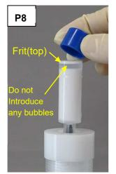
**Photograph P8**; assembly of the top blue cap on top of the frit and the settled bed in the column tube.
