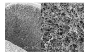
Fig 1. SEM analysis of Cellufine MAX base resin
