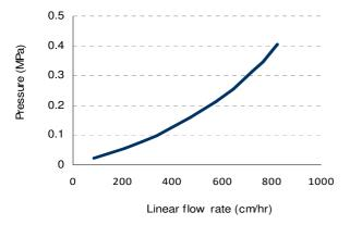
Figure 3. Pressure-flow velocity curves of Cellufine MAX GS (30 cm I.D. x 20 cm L), Mobile phase: Pure water at 24  $^{\circ}$ C.
