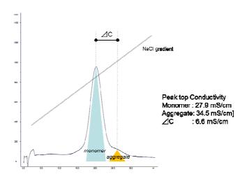
Figure 2. Mab Monomer/Aggregate Separation , Citrate Buffer (pH 5.0) NaCl:  $0.2{\rightarrow}0.5$  M ,Column: 5 mm I.D.  $\times$  50 mm L Mab: 1 ml injection , Flow: 0.66 ml/min [better to express as cm/h]
