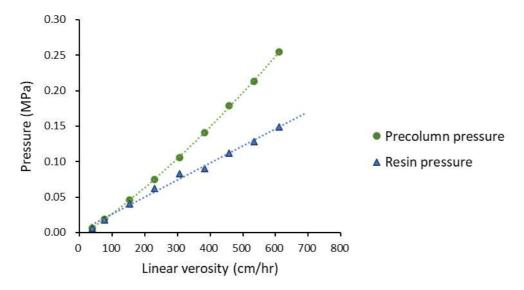
Column: I.D. 10 cm x H 20 cm Compression Factor: 1.30 Temp.: 24±1 °C Mobile Phase: Pure water
