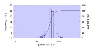
Fig. 3. Particle-size distributions of Cellufine A-500
