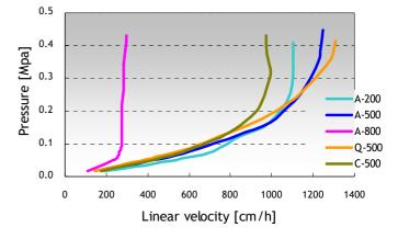
Fig 5. Pressure-flow velocity curves of Cellufine IEX media (2.2 cm I.D. x 20 cm L), Mobile phase with pure water at 24 °C,
