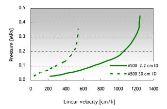
Fig 6. Pressure-flow velocity curves of Cellufine A-500 media (2.2 cm I.D. x 20 cm L and 30 cm I.D. x 20 cm L ), Mobile phase with pure water at 24  $^{\circ}$ C,
