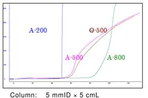
Column: 5 mmID × 5 cmL Flow rate: 150 cm/h Sample: 1 mg/ ml Buffer: 50 mM Tris-HCI (pH 8.5) for A-200, A-500 and A-800 50 mM Tris-HCI (pH 8.0) + 50 mM NaCI for Q-500
