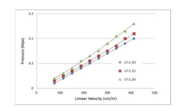
Figure 3, Pressure/Flow in a 3.2 cm ID column
