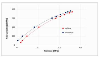
This data suggests that an optimal compression factor for packing Cellufine A-500 in a 30 cm ID column was 1.125 to 1.175. In Figure 4 above, a pressure - flow velocity curve of Cellufine A-500 packed in a 30 cm I.D. column is shown with flow in both directions.
