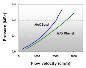
Fig 3. Pressure-flow velocity curves of Cellufine MAX Butyl and Phenyl (2.2 cm I.D. x 20 cm L), Mobile phase: pure water at 24  $^{\circ}$ C.
