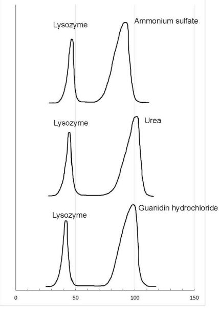
Column :  $1.6 \times 52$ cm (Vt = 104ml) Gel : Cellufine® G H - 2 5 Sample : 2 m I Lysozyme 30 m g/Salt 150mg Eluate : 0.05 M ammonium formate Flow rate : 42ml/hr (21cm/hr) Detection : R I
