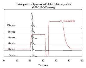
Cellufine Sulfate performance remains constant over at least 100 operating cycles. The data to the left shows 100 purifications cylcles follwed by cleaning in 0.5 M NaOH.
