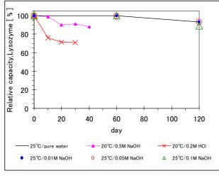
Fig2.Stability test in alkali and acid at  $20^{\circ}C/25^{\circ}C$ .
