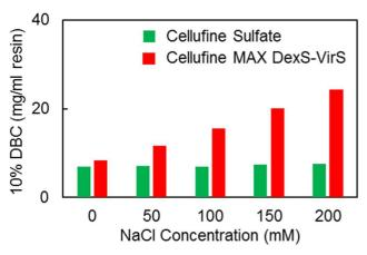
DBC was measured in a 5 mmID x 2.5 cmL (volume 0.49 ml) flow packed column at a flow rate of 0.125 ml/min for a residence time of 4 min. Lactoferrin at 2 mg/ml was loaded in a 50 mM Tris HCl buffer pH 7.5 + 0, 50, 100, 150 and 200 mM NaCl.
