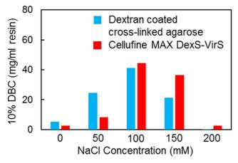
DBC was measured in a 5 mmID x 2.5 cmL (volume 0.49 ml) flow packed column at a flow rate of 0.125 ml/min for a residence time of 4
