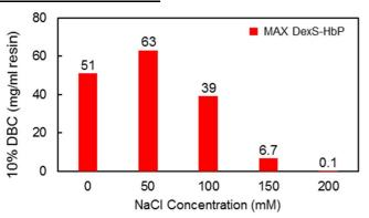
DBC was measured in a 5 mmID x 2.5 cmL (volume 0.49 ml) flow packed column at a flow rate of 0.125 ml/min for a residence time of 4 min. Polyclonal IgG at 2 mg/ml was loaded in a 10 mM Na Acetate buffer pH 5.0 + 0, 50, 100, 150 and 200 mM NaCl. A more extensive study looking at both salt and pH variables is summarized in Table 2, below.
