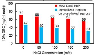
DBC was measured in a 5 mmID x 2.5 cmL (volume 0.49 ml) flow packed column at a flow rate of 0.125 ml/min for a residence time of 4 min. Lactoferrin at 2 mg/ml was loaded in a 10 mM Na Phosphate buffer pH 7.5 + 0, 50, 100, 150 and 200 mM NaCl.
