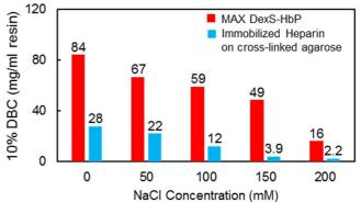
DBC was measured in a 5 mmID x 2.5 cmL (volume 0.49 ml) flow packed column at a flow rate of 0.125 ml/min for a residence time of 4 min. Lysozyme at 2 mg/ml was loaded in a 50 mM Tris
