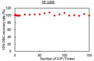
Protein recovery after multiple cycles of base CIP was measured in a 5 mmID x 2.5 cmL (volume 0.49 ml) flow packed column at a flow rate of 0.125 ml/min for a residence time of 4 min. Lysozyme at 2 mg/ml was loaded in a Buffer A; 50 mM Tris HCl pH 9.5 + 150 mM NaCl. Retained protein was recovered by elution with Buffer B; 50 mM Tris HCl pH 9.5 + 1.0 M NaCl.
