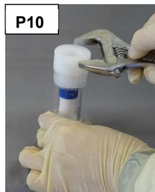
**Photograph P10;** Using an adjustable wrench to seal top screw
