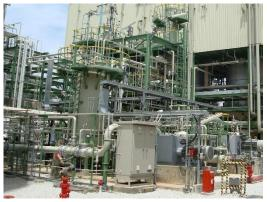
The un-reacted VCM gas in the gas holder is compressed and condensed in the recovery section. The recovered liquid VCM is stored in a vessel and is reused as the feedstock for the succeeding polymerizing reaction.
