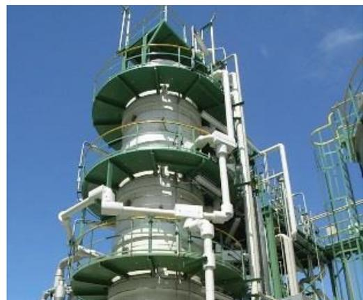
The PVC slurry in the slurry tank is fed to stripping column, where the un-reacted VCM is effectively stripped out from the slurry with steam and stripped slurry is transferred to the drying section. The final VCM content in PVC is less than one (1) ppm. The VCM Removal system uses heat exchanger to minimize the steam consumption. The hot water is used as washing for each stage inside the stripping column. This contributes to continuous operation for a long term without stopping
