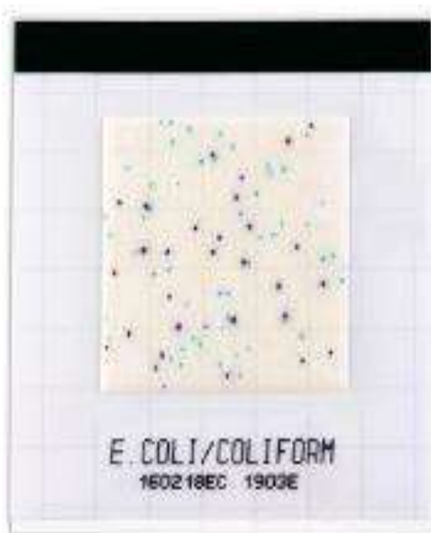
Picture 1: Typical colonies on JNC Media Pad EC: Blue/Green = coliforms Red/Navy = E.coli
